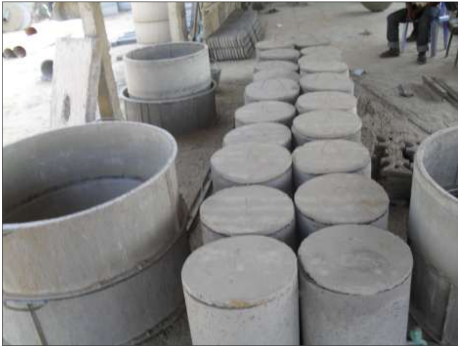
Concrete latrine pit liners
